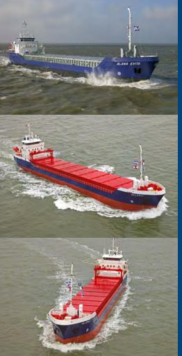
The Bijlsma trader 3250 is the true multipurpose vessel in the range of Bijlsma shortsea vessels. Equipped with a tanktop strength of 20 tons per square meter, the vessel is specifically designed to carry heavy bulk cargos.
